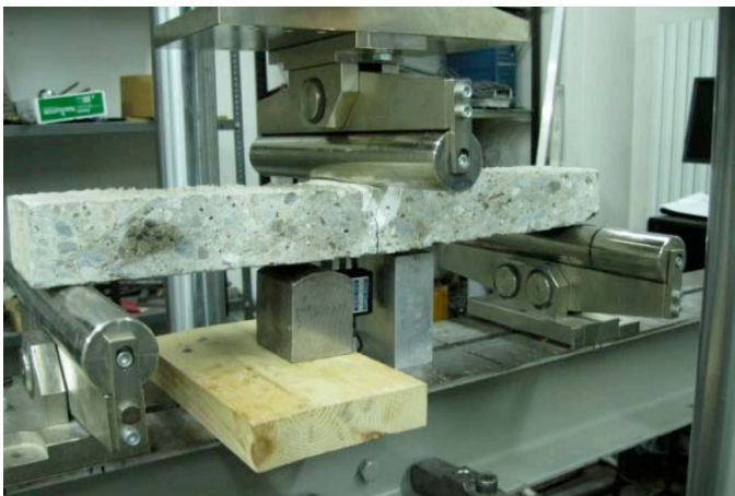
Figure 2: 3-point bending test set-up
