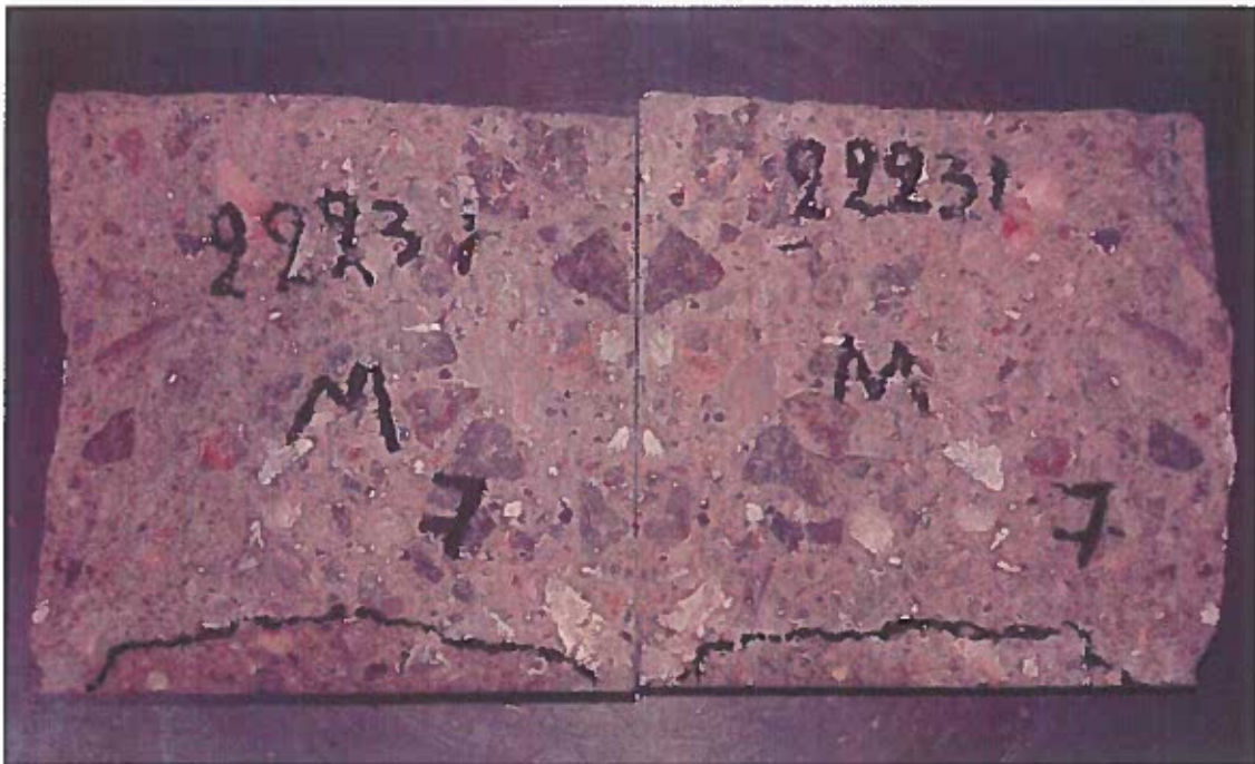
Picture 5. 22231-07 specimen (Witness) – After the end of the 4 th week
