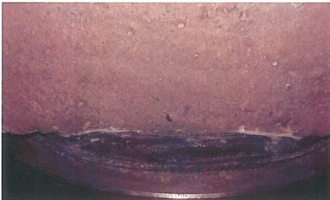
Picture 4. 22231-01 specimen (With PENETRON ADMIX) – After the end of the 4 th week – Generation of crystals
