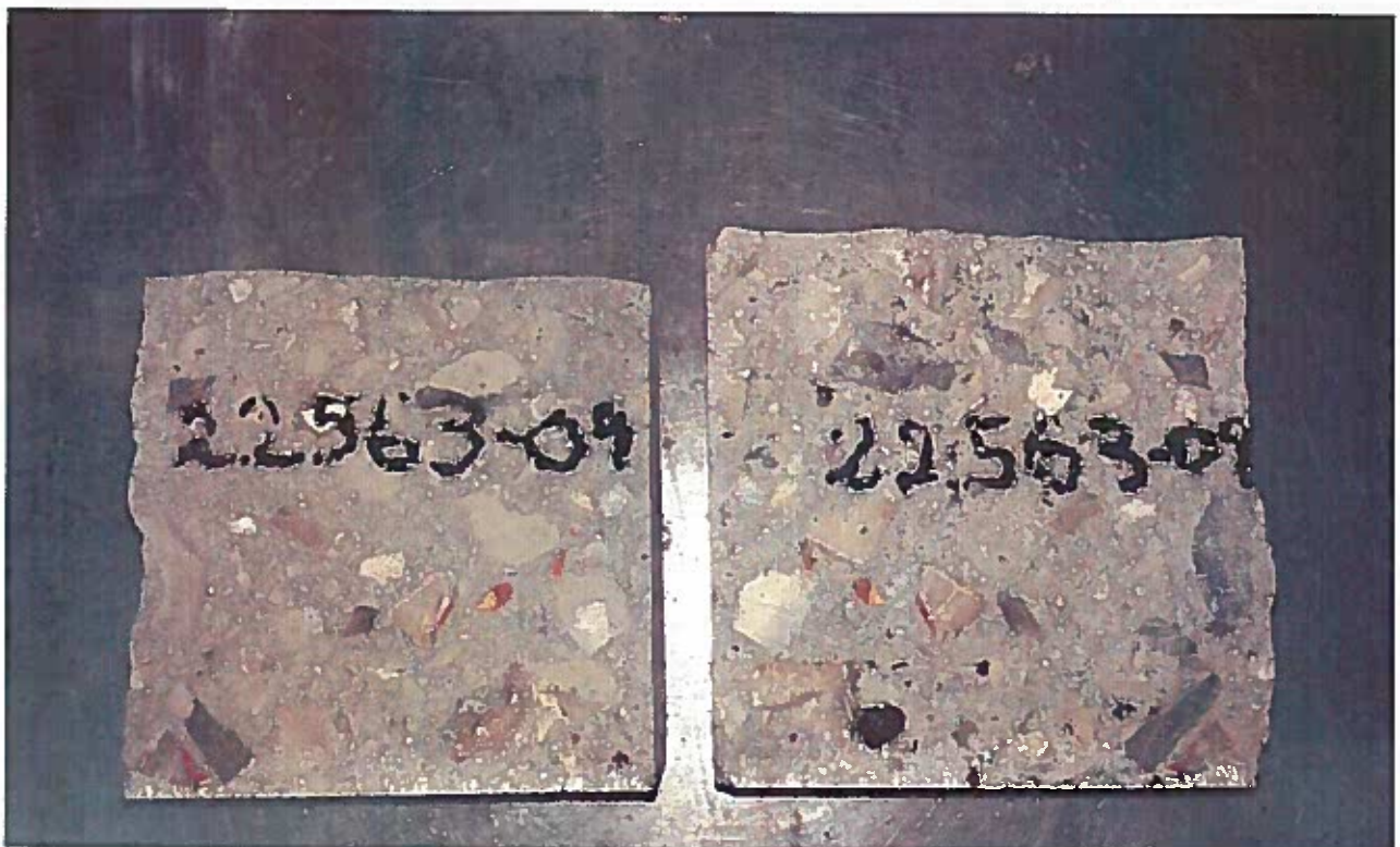
Picture 2. 22563-09 specimen (With PENETRON ADMIX) – After the end of the 4 th week
